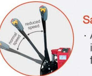
Automatic braking when the handle is either perpendicularly pulled or fully lowered
