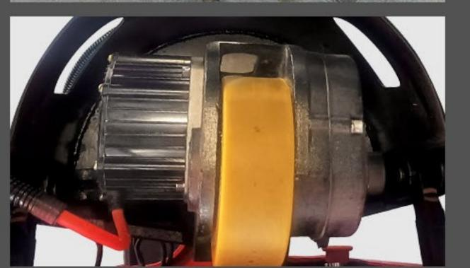
800W big power motor, strong power, low energy consumption DC permanent magnet driving motor, strong power and long service
