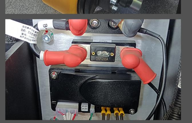
Curtis solid state controllers provide smooth acceleration and seamless directional control. Its regenerative braking feature adds energy back to the battery to improve efficiency.
