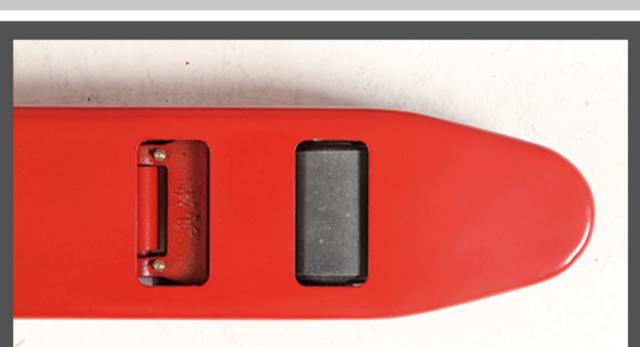
Entry rollers prevent physical exertion of the operator and protect load rollers and pallet.
